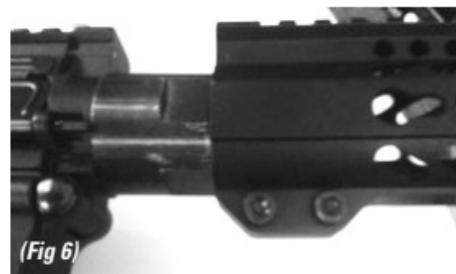
**STEP 7.** Loosen Handguard Retainer Screws and slide Handguard over Barrel Nut. (Fig 6)
