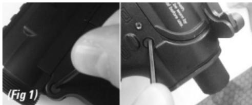
**STEP 2.** Split T15™ by releasing the front and rear strip pins. (Fig 1)
