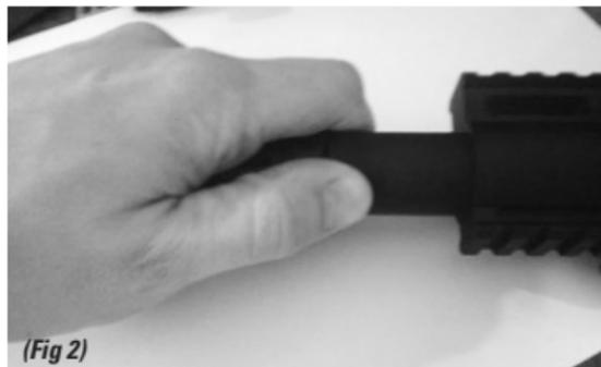
**STEP 3.** With the magazine removed rotate the barrel by grabbing it at the end between the muzzle brake and the gas block. Look into the magazine well to confirm the position of the ball port in the barrel. **DO NOT** try to rotate the barrel by rotating the Handguard or gas block. This will cause damage to your marker. The barrel should slide out with very little force. (Fig 2)
