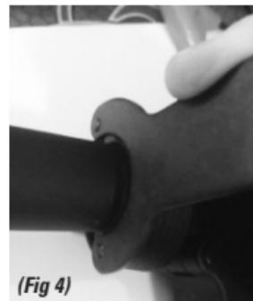
**STEP 5.** Take the 4 point Handguard off of the marker and use the Spanner Wrench tool to remove the barrel sleeve. (Fig 4)
