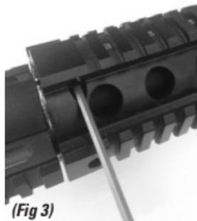
**STEP 4.** Remove stock 4 point handguard by accessing the 4 hex screws using the size 3 metric hex key on the top of the handguard. (Fig 3)
