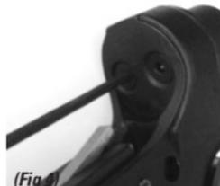
**STEP 4.** Remove stock ASA using 1/8" hex key. Keep stock ASA screws and mounting screw o-ring for installation of your Remote Buffer Tube Adapter. (Fig 4)
