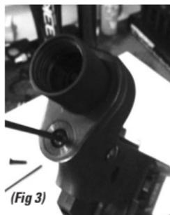
**STEP 3.** Remove Rear ASA Port using 3/32" hex key (Fig 3)
