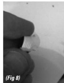
**STEP 8.** Apply teflon tape to the 1/8NT Threaded Plugs and place in the 2 unused ports. (Fig 8)
