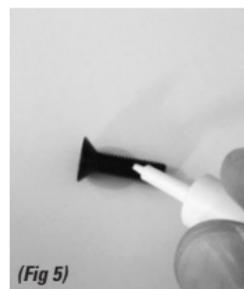
**STEP 5.** Clean off stock ASA screws and apply blue thread locker. (Fig 5)
