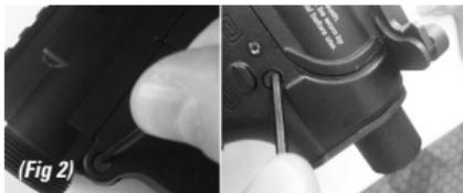
**STEP 2.** Split T15™ Upper Receiver from the Lower Receiver by pushing out the front and rear trip pins. (Fig 2)
