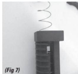
**STEP 7.** Place spring on follower inside magazine extender and compress spring and follower into magazine extender. (Fig 7)
