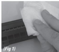
**STEP 1.** Wipe down FSC body and remove any mud, debris, or paint residue from the unit. (Fig 1)
