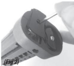
**STEP 2.** Using screw driver or o-ring pick, remove magazine end cap, exposing the stock magazine spring and follower. (Fig 2)
