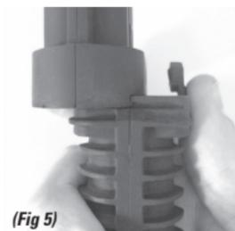
**STEP 5.** Install FSC magazine extender by placing extender on magazine end cap rail like so. Extender should slide on FSC magazine without force. (Fig 5)
