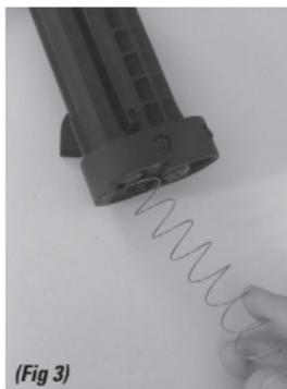
**STEP 3.** Remove stock spring from FSC magazine. (Fig 3)
