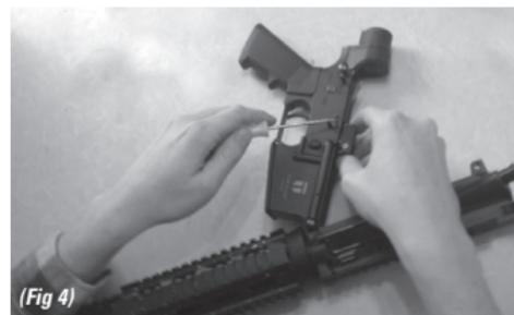
**STEP 5.** Remove stock Semi-Auto Trigger group and for creating accessibility, remove Upper Manifold (fig 4)
