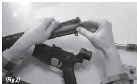
**STEP 3.** Remove old Bolt assembly and Striker Buffer. (fig 2)
