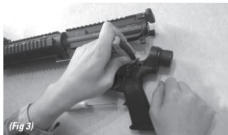
**STEP 4.** Remove Selector Switch by pressing down on opposite side of Selector Switch. If selector switch does not pop out, remove AR grip by using 7/32 Allen Key. (fig 3)
