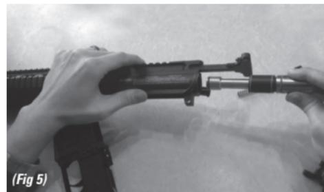
**STEP 6.** Install High-Flow Bolt and new striker spring, and Full-Auto Striker Buffer (included in packaging) (fig 5)
